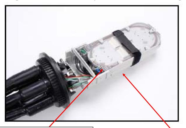
Hinged Tray (2533) which accommodates 24 single fusion, 12 mechanical, or 48, 72, 80, or 120 mass fusion splices (4-, 6-, 8-, or 12-fiber ribbons); maximum # of trays = 2
