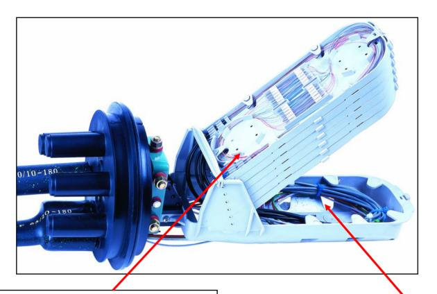
Hinged Tray (2533) which accommodates 24 single fusion, 12 mechanical, or 48, 72, 80, or 120 mass fusion splices (4-, 6-, 8-, or 12-fiber ribbons); maximum # of trays = 6
